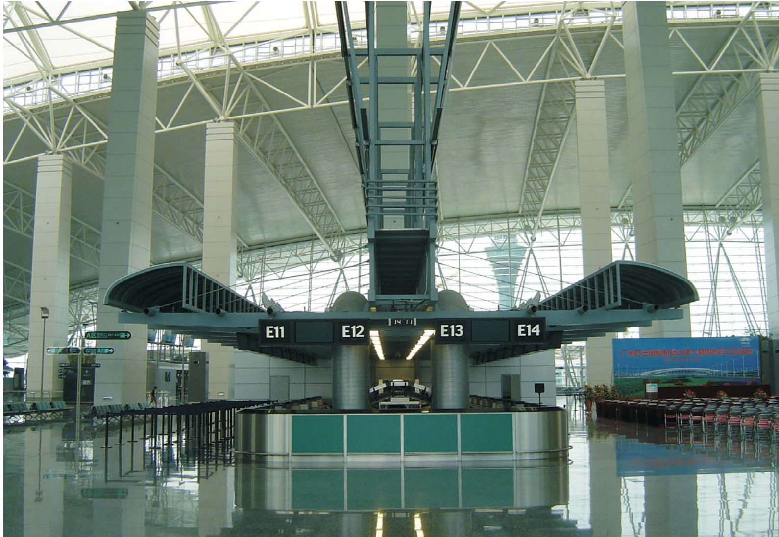
Guangzhou-Check-in island head; powder coated Mild steel, with Aluminium cladding
